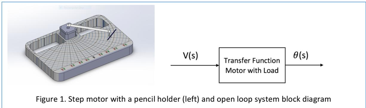
Figure 1. Step motor with a pencil holder (left) and open loop system block diagram
