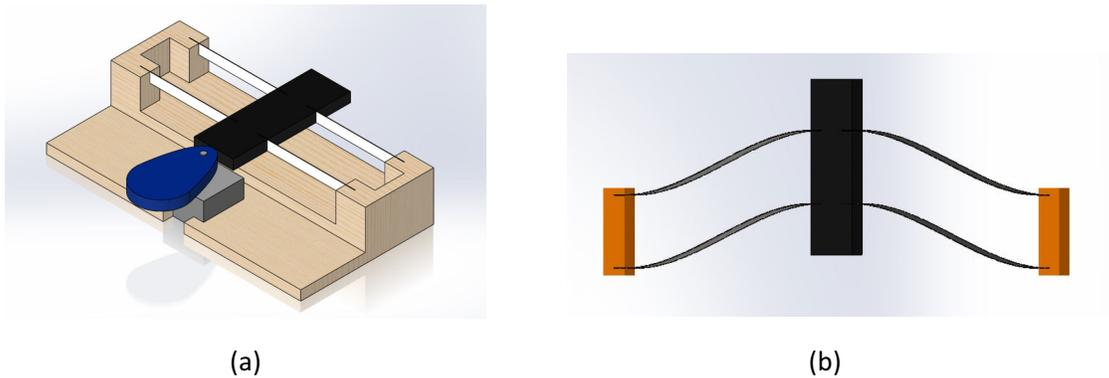
Figure 2. (a) Flexible double arm as alternative to rigid slider crank mechanism, (b) The deflected configuration of the flexible beams
