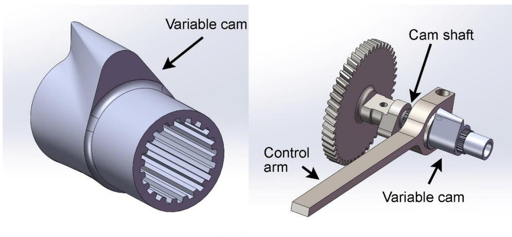
As shown in the figure above, the variable cam slides along the splined cam shaft. In the figure above on the left, an enlarged view of the variable cam is seen.
