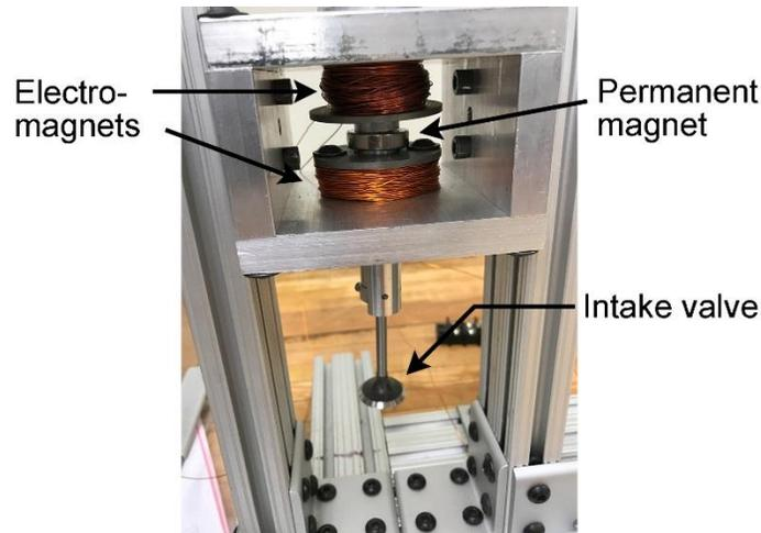
The permanent magnet is fixed to the shaft of the intake valve. The permanent magnets have reverse polarity, and are turned on and off by a signal from a computer that is synchronized to the engine speed. The electromagnets cause the permanent magnet to “pop off” the iron core of the electromagnets and move to the opposing side. The rpm and power of the engine is determined by how long the valve is open on the intake stroke of the engine.
