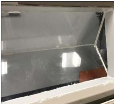
Figure 2: The four acrylic plates used to cover the foam layer.
