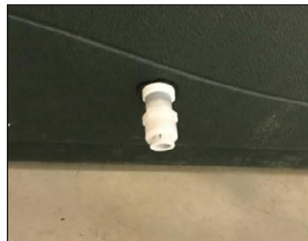
Figure 6: Exterior view of assembled bulkhead fitting for pressurized air supply to nozzle.
