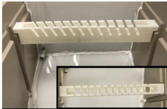
Figure 7: 3-D printed specimen holder (ABS plastic)
