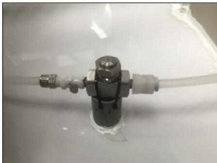
Figure 5: Assembly of the nozzle and nozzle tower. Solution feed is on the left side of the nozzle and air feed on the right.
