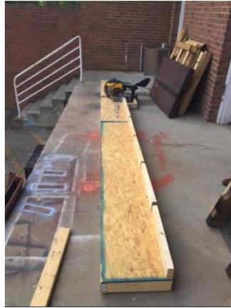
Figure 2: De-nailing jig
