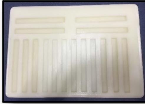
Figure 1: Rubber mold used for manufacturing epoxy specimens
