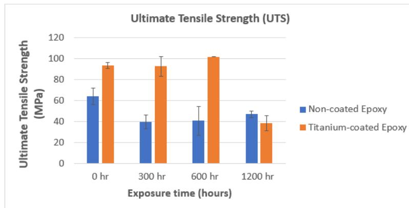
Figure 4: The ultimate tensile strength of epoxy and titanium coated epoxy after 0, 300, 600 and 1200 hours of exposures
