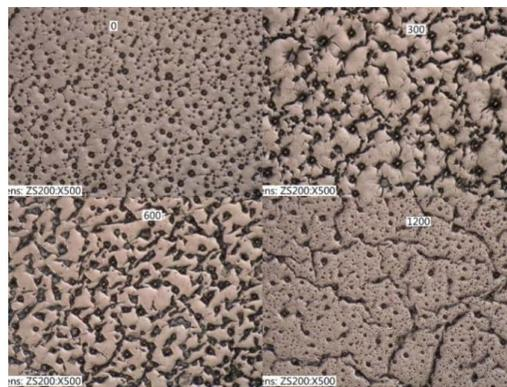
Figure 3: Optical microscopy images of titanium coated epoxy after 0, 300, 600 and 1200 hours of exposure (500 X magnification)
