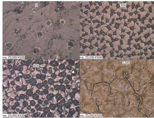
Figure 2: Optical microscopy images of epoxy surface after 0, 300, 600 and 1200 hours of exposure (500 X magnification)
