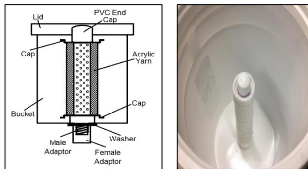
*Figure 1. DIY Filter Design and Prototype*
