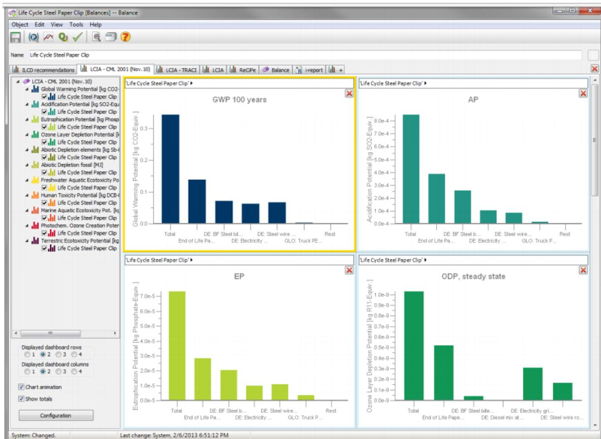
Figure 3. GaBi Life Cycle Impact Analysis Result Screen
