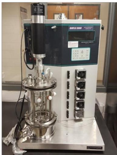
**Figure 1.** Bioflo 3000 5 L Benchtop Bioreactor.
