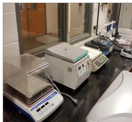
**Figure 3.** (From Left to Right) Incubator/Shaker, Centrifuge, Heated Stir Plate, Spectrophotometer, Mini Centrifuge, and Pipettes.
