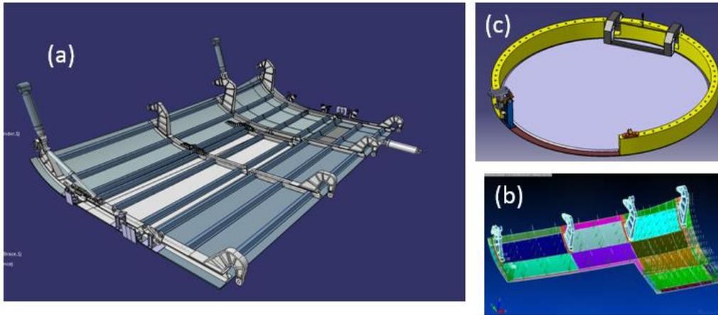
Figure 3. Student design of main landing gear door for (a) Airbus A380, (b) corresponding finite element analysis and (c) design for Boeing 737.
