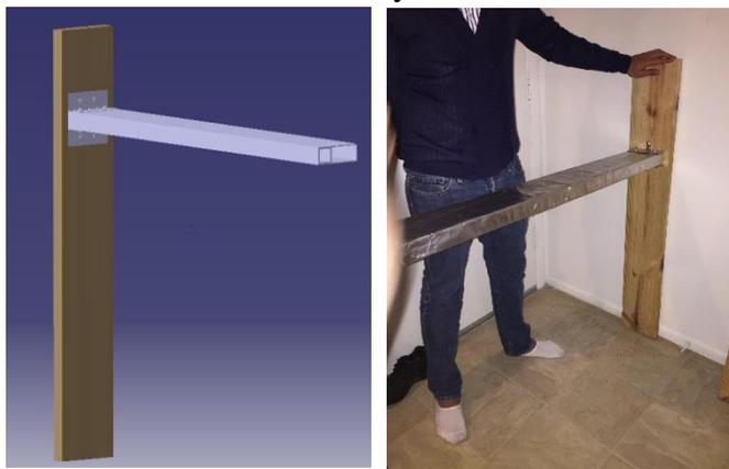
Figure 1. Design and fabrication of cantilever beam using aluminum foil for the mini-project.
