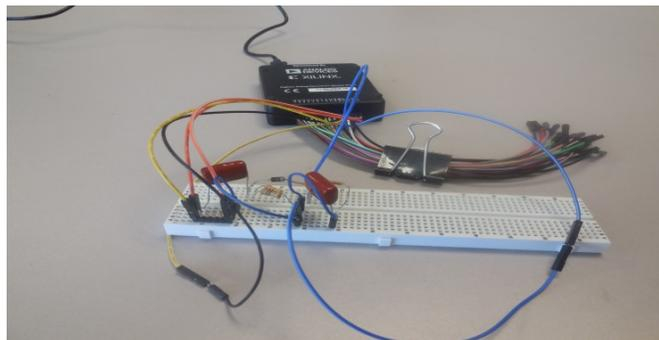
Fig. 5: FM Demodulator breadboard
