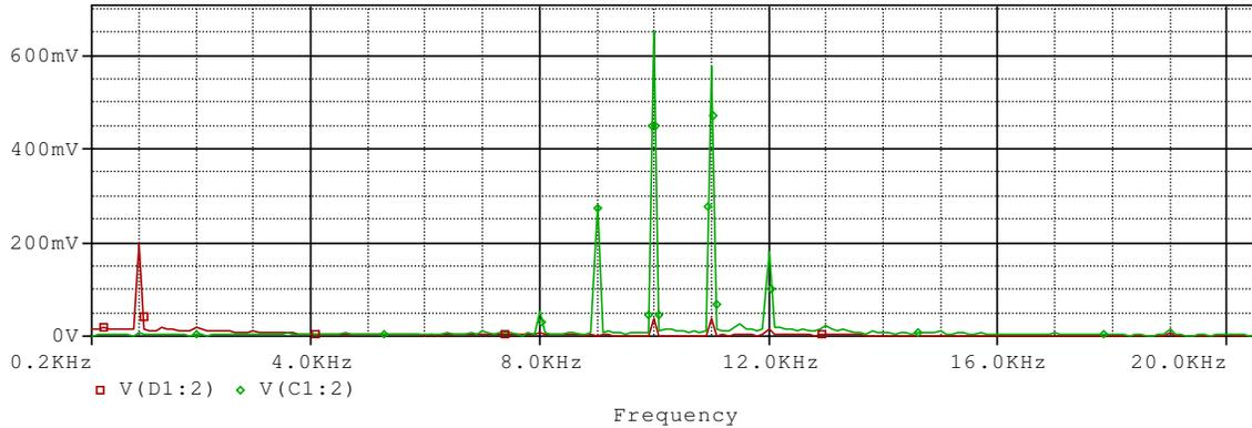
Fig. 4: FFT measured at V3 in demodulator circuit for  $\beta = 0.1$ . The 1 KHz demodulated output is shown in red.
