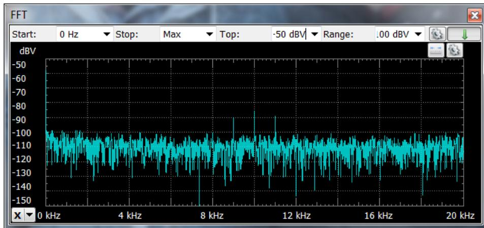
Fig.7: FM demodulator signal measured at the diode input using the Analog Discovery system.
