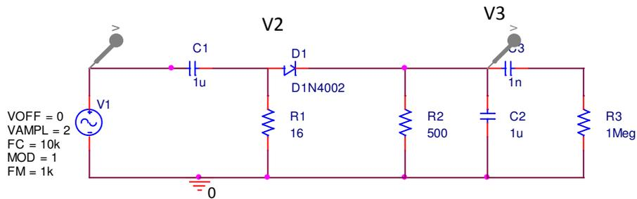
Fig. 3 FM Demodulator Simulation
