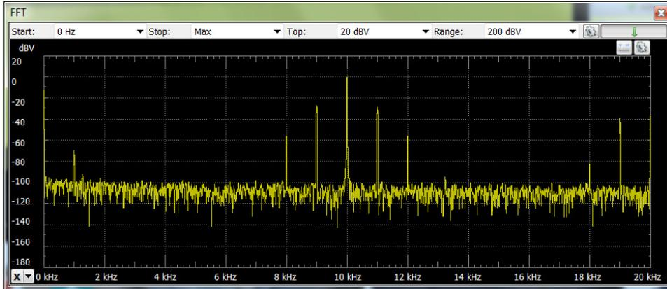
Fig. 6: FFT of the FM input signal generated using the Analog Discovery system.
