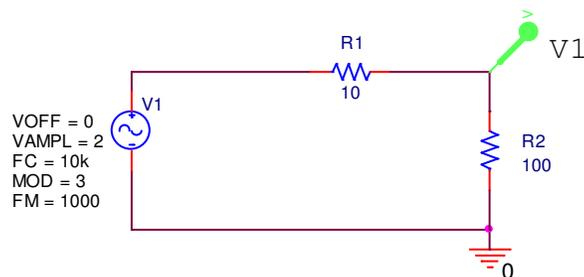
Fig. 1 FM Modulator Simulation
