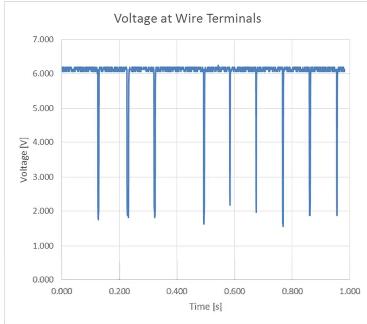
Figure 2: Simple DC motor battery voltage vs. time for determining motor speed.
