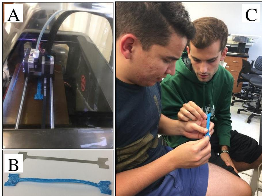
**Figure 2:** (A) A prototype sample coupon being 3D printed in PLA. (B) A Finished 3D printed coupon compared against an aluminum original upon which it is based. (C) Students evaluate the print quality and tool path of the coupon as they iterate to improve its design.
