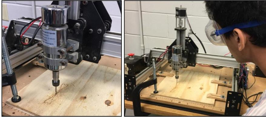
**Figure 3** (Left) Testing router tool paths in wood in preparation to cut a coupon from plastic sheet. (Right) A student watches the router path to ensure no tool crashes during sample fabrication.
