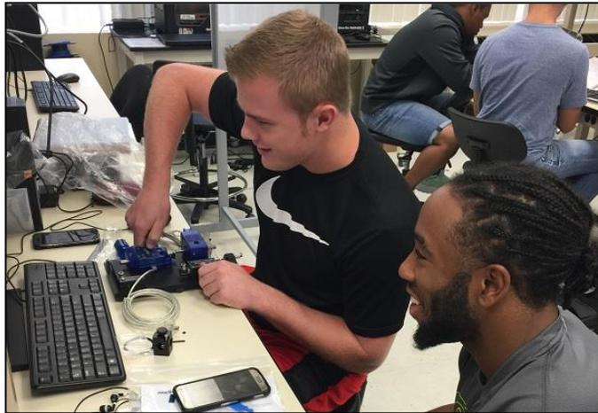
**Figure 1:** Students learn how to use the PASCO EX-5515A stress-strain apparatus in preparation to designing and fabricate new test samples for the educational lab device.
