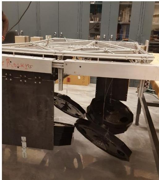
**Figure 1. G-Loading test shows temporary deflection after 370 lbs. were suspended from the rig at the Structures Lab in the College of Engineering (CoE).**
