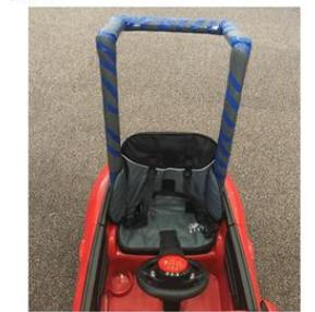
Figure 2. Support system for Daijah's vehicle.
