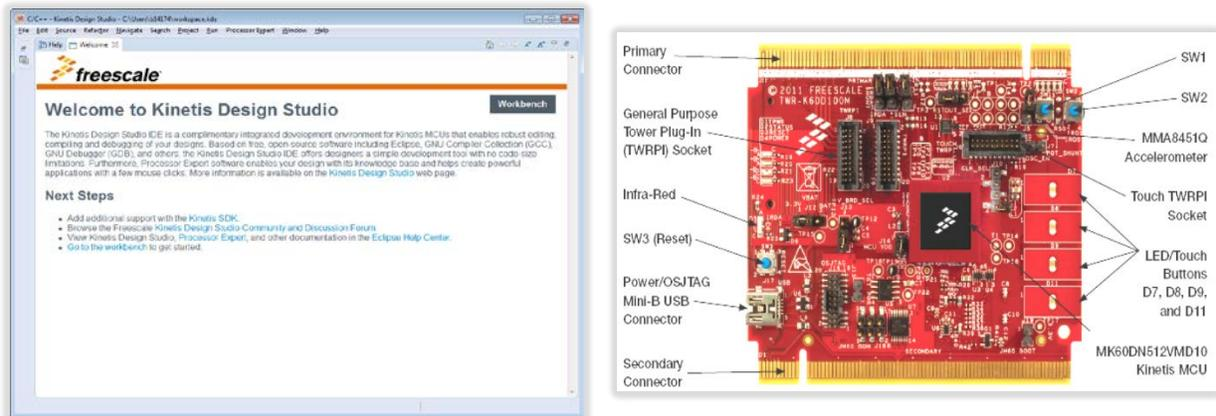
Figure 4: Implemented KDS IDE and TWR-K60D100M Development Board.
