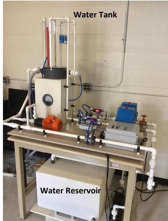
Figure 1. Water tank experiment. Pumps circulate water from bottom reservoir (below table) to tank above.
