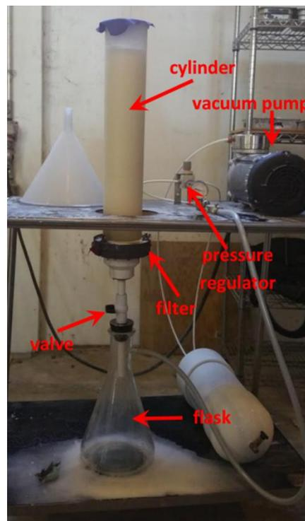
Figure 2. Batch filtration experiment.
