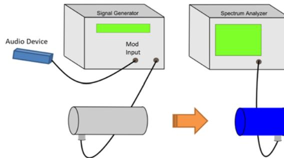
**Fig. 1.** Demonstration setup. An audio signal is sent from one side of the room to the other.
