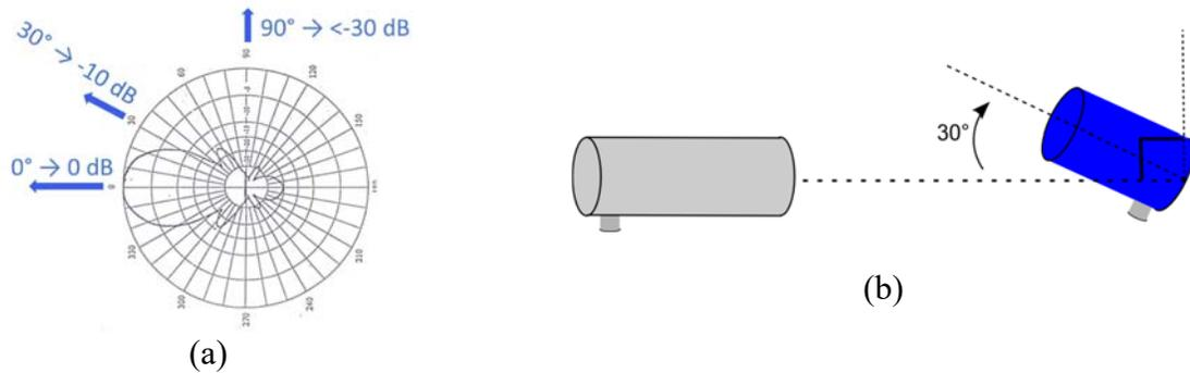
**Fig. 2.** (a) E-Plane radiation pattern of the tube antenna (P2412)<sup>8</sup>. (b) Angle of rotation of the receiver's antenna.
