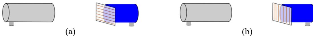
**Fig. 4.** Positioning of the wire grid polarized on the receivers antenna.
