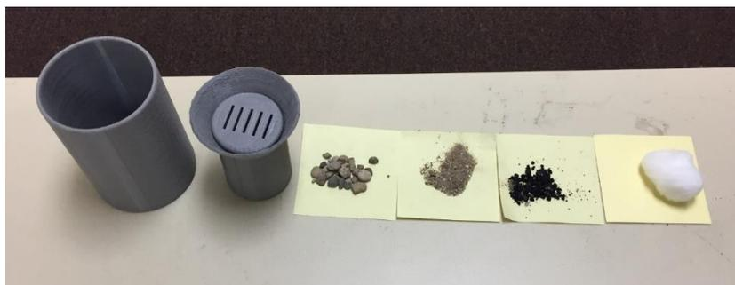
Figure 2: Prototype of 3d Printed Smart Cup (cup, filtering cartridge, and lid) and filtration materials (gravel, sand, granular activated carbon, and cotton wool).
