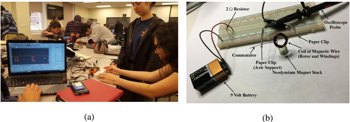
Figure 5 (a) Electric Motor Mini-project. (b) Motor details
