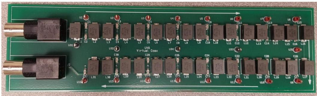
Figure 2 Artificial Transmission Line
