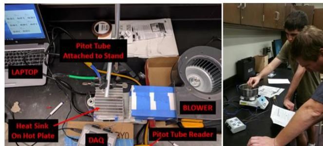
Figure 2. a) Lab 5 experimental configuration and b) students conducting Lab 4.
